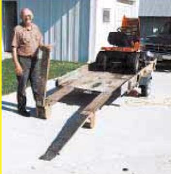
when we folded the full-length ramps straight up after loading, the wind would catch them when we were driving. So we cut the ramps exactly in half and installed hinges to allow them to fold. To reinforce them at the hinge point, we made a couple supports out of plywood. They fasten to the ramps just ahead of the hinge point.
