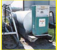
tion gas pump mount on a pair of large steel skids. It can be used on the farm for normal refueling or taken to the field. (C.F. Marley, Nokomis, III.)
