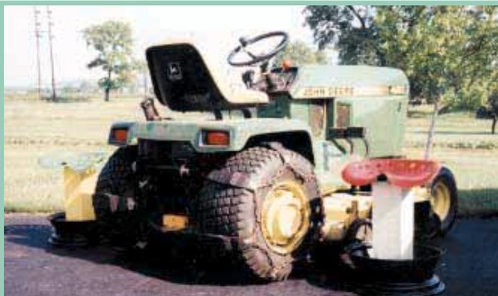
I made "chains" for my garden tractor out of rubber tires. I just cut strips out of a car tire and bolted them to lengths of chain that wrap around the sides of the tire. The rubber strips are a couple inches wide and lay flat on the tire, giving you extra traction without ripping up the ground. Great on steep hillsides when
