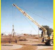
der pulls up on the center hinge of the bucket. A pair of chains run from the bucket to the boom truck to keep it from swinging too much. This has worked great for me for all these years. (Eugene M. Durand, 5404 Ocotillo, HC 31, Box 1020Z, Roswell, NM 88201)
