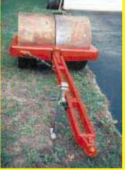
king pin, welding a 6-ft. drawbar to the kingpin. I used a 2 5/16-in. ball hitch to add flexibility when towing. I put a ratchet jack from the yoke to the drawbar to enable us to offset the roller to reach past the tractor wheel. The roller wheel is 50 in. wide and 40 in. high. (George Wojnar, 5 Malsbury Lane, Cream Ridge, N.J. 08514 ph 609 758-7295)
