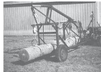
**Reeks's log hauler straddles the log. Two sets of hand-powered log tongs lift it on the highway.**
