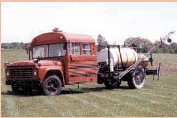
Beer cut off part of bus and mounted a 700-gal. fiberglass tank on frame. Note tall 38-in. tractor tires on back.
