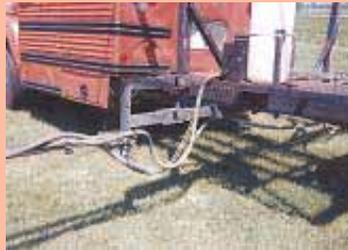
He used 2-in. sq. tubing to make the boom, which has a 1-in. tube behind it where nozzles mount.
