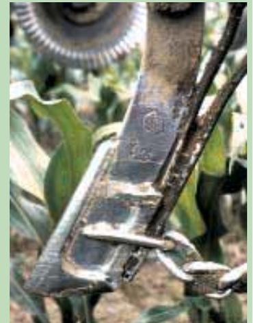
Photo shows how chain attaches to shank. Note two anhydrous tubes on knife.
