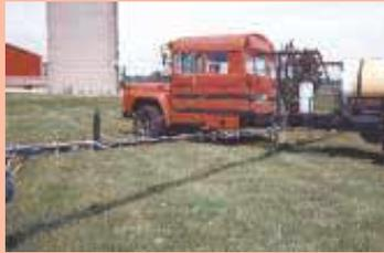
Each boom section mounts to frame with a hinge that's made so he can position boom sections at three different heights. Note 300-gal. water tank on frame.
