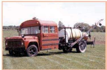
Beer cut off part of bus and mounted a 700-gal. fiberglass tank on frame. Note tall 38in. tractor tires on back.
