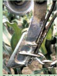
Photo shows how chain attaches to shank. Note two anhydrous tubes on knife.
