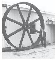
Winter stands beside a 12-ft. dia. rope pulley off a 150 hp. steam engine. At one time it was used by a grain elevator to run a generator, grain mill, and line shaft.
