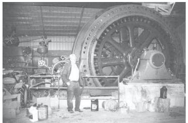
Perhaps the most unusual collectible in the museum is this 100-ton electric power plant. The steam-powered engine has an armature flywheel that's 16 ft. in diameter.
