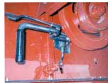
Steel brackets bolt to each side of combine and come with linkage that attaches to rear bolt of tray.
