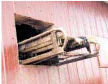
Top end of conveyor sticks through opening in barn wall. As Hering cleans the pens, he throws manure and used bedding onto conveyor and it's emptied into a spreader outside.
