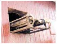
Top end of conveyor sticks through opening in barn wall. As Hering cleans the pens, he throws manure and used bedding onto conveyor and it's emptied into a spreader
