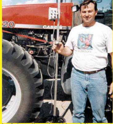
Larry Bearinger says his company's new "wireless controller" lets you operate the throttle and hydraulics on any tractor by remote control. "It works great for operating pumps and pto's from far away," he notes.
