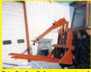
Extending the cylinder causes arm to push bale off. Unit can be used on a front-end loader or 3-pt. to load bales into feeder rings.
