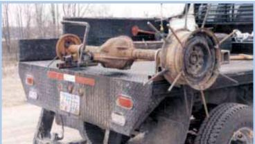
Wire roller bolts to truck flatbed. It consists of a car rear end with a wheel and rim attached to one of the hubs. Lengths of 6-in. rebar are welded to each side of rim.
