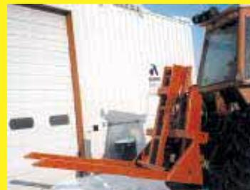
Loader's 4-ft. long push-off arm is operated by a big hydraulic cylinder. With cylinder in retracted position the arm is straight down.
