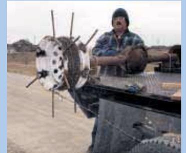
A crank welded onto the rear end's input shaft is used to turn the wheel.
