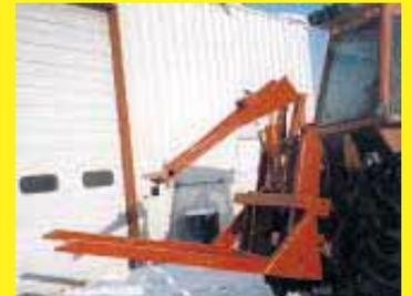
Extending the cylinder causes arm to push bale off. Unit can be used on a front-end loader or 3-pt. to load bales into feeder rings.
