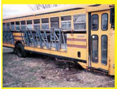
Multiple self-locking headgates cover holes cut into side of bus. After driving out to pasture, Kerr dumps grain onto floor in front of each headgate to catch cows.
