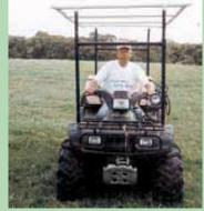
"Sun roof" is made from a PVC frame covered by a close-weave fiberglass cloth. tank and from having no support.
