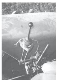
Davies uses a "joystick" to control the extra hydraulic outlets.
