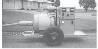
Olson made generator trailer from the front axle of a 3/4-ton pickup.
