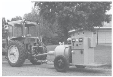
Ellsworth Olson and Meredith Ulstad converted a 100 hp, 3-phase synchronous electric motor into a pto-powered backup generator.
