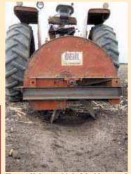
He cut off about a third of the blower and then built a heavy angle iron frame around it. Blower fan digs a shallow ditch about 20 in. wide and 5 to 6 in. deep at center.
