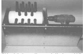
Chicken plucker is powered by any standard hand-operated drill.
