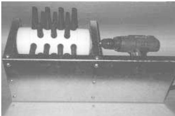
Chicken plucker is powered by any standard hand-operated drill.
