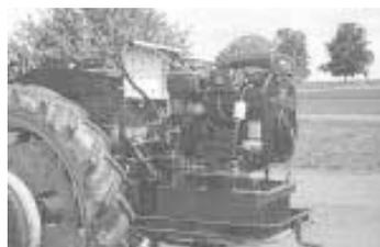
original Continental engine is no longer made and parts for it are no longer available. I use this tractor a lot to clean my barn and for other jobs, having built a front-end loader for it years ago. I didn't want to give it up so I removed the engine and replaced it with a new Kohler 2-cyl., 25 hp, air-cooled gas engine. It works great.
