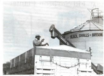
Remote auger "shut-off" lets you finish leveling off your truck without having to climb down to shut off augers.
