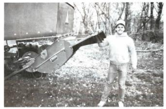
Hinge kit lets you fold straw chopper down out of way when not needed or swing it back up for use. Spring latch holds it in place until you can install mounting bolts.
