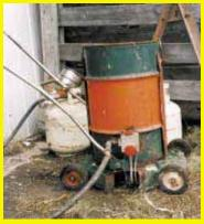
ing element from a gas water heater mounts in the bottom of the barrel. I converted it from natural gas to propane by drilling out the orifice (or you can buy a new fitting). The water heater thermostat keeps the water right at 140 to 145°, which is perfect for scalding birds. (W.K. Rynsburger, RR2, Site 23, Box 7, Grande Prairie, Alberta T8V 2Z9 Canada ph 780 532-6566)
