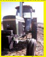
to see where you're going. Besides seeing auger hoppers or front-mounted equipment, you can also see disk marks and obstacles in the field. Almost any kind of light can be mounted on the side of the tractor on almost any kind of bracket. This 4440 has an extra light just above the front axle and a couple feet behind the axle. (Mark Mahlow, 71573 120th St., Zearing, Iowa 50278 ph 515 487-7708)
