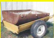
tailgate on back that can be opened and closed. The trailer dumps to the back, pivoting on the axle. You can dump it manually or I also use a small boom that mounts above the trailer tongue to dump it. I use the other half of the tank to mix concrete and motar. I've even used it as a boat in my pond. (Bill Reeks, 7104 U.S. Hwy 231 N, Cromwell, Ky. 42333)
