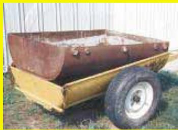
tailgate on back that can be opened and closed. The trailer dumps to the back, pivoting on the axle. You can dump it manually or I also use a small boom that mounts above the trailer tongue to dump it. I use the other half of the tank to mix concrete and motor. I've even used it as a boat in my pond. (Bill Reeks, 7104 U.S. Hwy 231 N, Cromwell, Ky. 42333)
