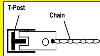
that will fit over the back side of a post. Then bend a second piece of steel into a U shape to fit around the front side of the post. It should be long enough to weld about 1 in. on each side to the first part of the puller. There should be enough space to fit down over a standard T post.
