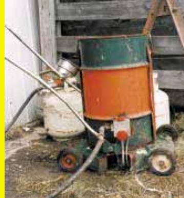
ing element from a gas water heater mounts in the bottom of the barrel. I converted it from natural gas to propane by drilling out the orifice (or you can buy a new fitting). The water heater thermostat keeps the water right at 140 to 145°, which is perfect for scalding birds. (W.K. Rynsburger, RR2, Site 23, Box 7, Grande Prairie, Alberta T8V 2Z9 Canada ph 780 532-6566)
