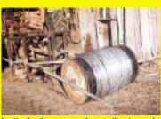
I attached a garage door pulley to each end of a 55-gal. drum to wind up electric fence wire. The drum mounts on a couple "arms" made out of angle iron that attach to a 3-pt. mounted forklift. I can wind up wire as fast as I can drive my tractor in the pasture. I made the angle iron arms extra long to keep the wire from going off the ends of the barrel. This works well. (Bill McSherry, 4569 SW Hwy. 166, Columbus, Kan. 66725 ph 316 674-3332)
