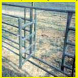
36-in. wide opening. The top and bottom bars were not cut out. Two vertical braces were cut out of 2-in. dia. lightweight conduit. The hinges are made out of two 8-in. long pieces of 3/8-in. round stock set into 3/8-in. collars. The latch was also made using a piece of 3/8-in. round stock with a couple collars and a spring.
