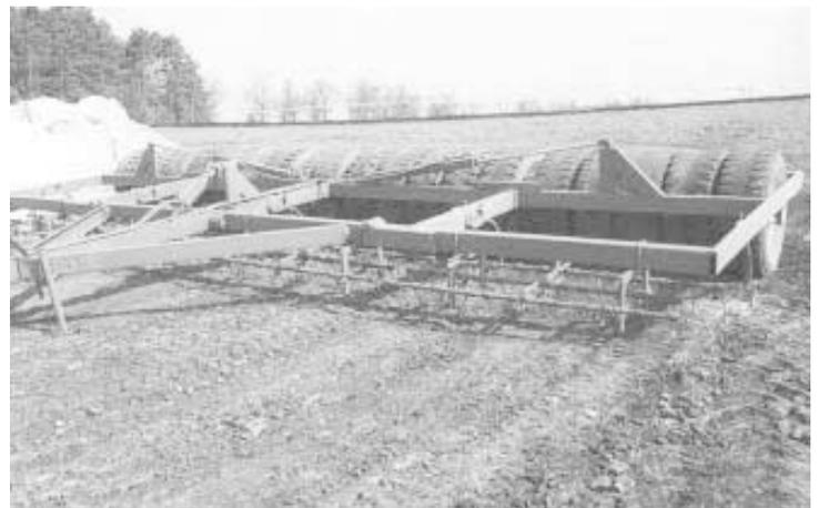
**Packer consists of four sections of tires - two at center with a wing section at each end.**
