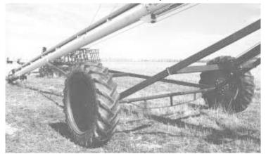
Big tractor wheels raise working height of auger, eliminating the need to build up under the wheels at the bin site.
