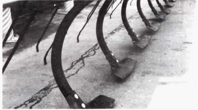
The square-bladed shovels hit weeds "dead on" and never get any narrower as they wear.
