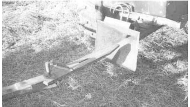
**Schreyer's hitch consists of a receiver "cone" on the tractor and a pivoting hitch bar that pins to front of wagon tongue. Hitch bar has a slot in it.**
