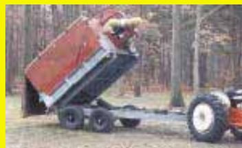
Box on tandem axle trailer measures 6 by 8 ft. inside. It's raised by a 3,000-lb. lift hoist which runs off a 12-volt battery.
