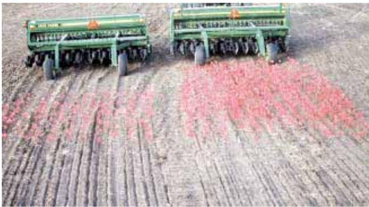
These two Deere 750 drills were pulled out of the ground at the same time. Drill on the left was equipped with the Seed Mizer attachment; the drill on the right did not have it. Flags mark seed left on the ground by each drill. There are 1,490 flags on the right but only 452 flags on the left.
