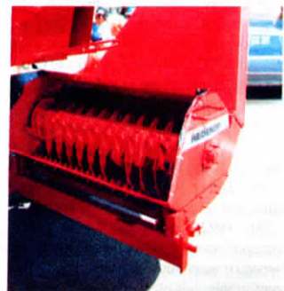
Chopper hinges outward to allow easy access to back of combine. Can be fitted with either spreader fins or a load-out chute (pictured) which lets you load chopped residue into a trailing wagon.
