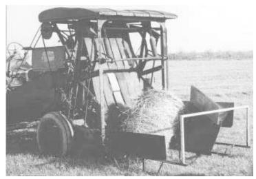
The brothers built a skid-mounted bale "straightener" that tows behind the AC baler.
