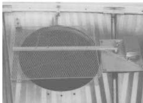
“Lifesaver 2000” installs on underside of bin roof. It consists of an expanded metal screen that covers the bin opening.
