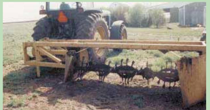
This pull-type composter was built out of a Howard Rotovator and is equipped with a 20-in. dia. beater. He used the same design on self-propelled composter shown above.
