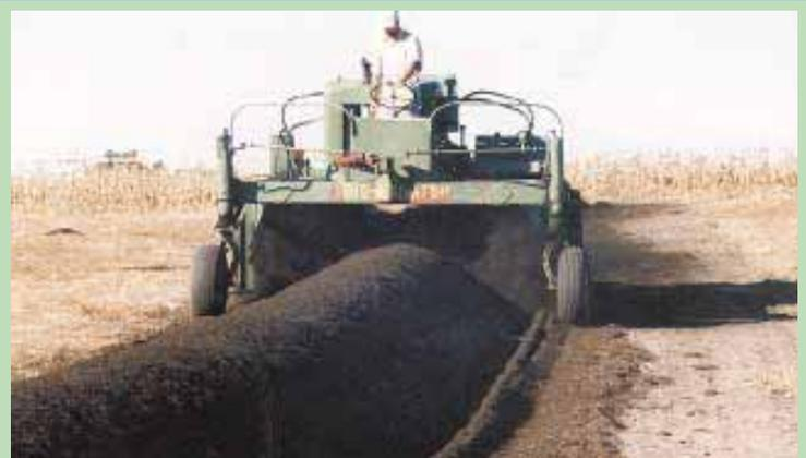
Soda built this self-propelled composting machine by rebuilding a Highboy sprayer.
