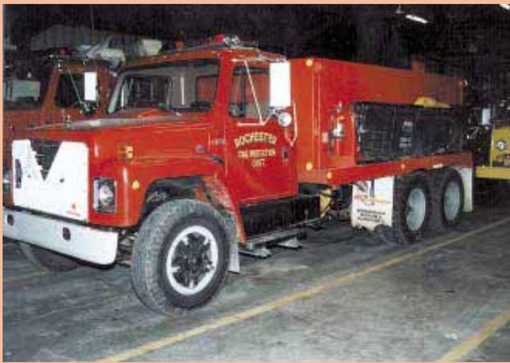
Fire truck is designed so it can be pulled forward while the water hose is working to move with the blaze.
