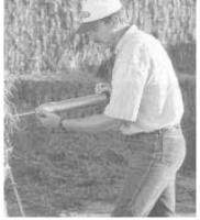
Hay sampler has an easy-to-use "push-in" probe that cuts a core 5/8-in. in diameter and 18 in. long.
