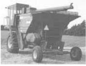
To double the size of the grain tank, he cut the back out and extended it out over the rear axle
