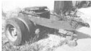
Trailer is fitted with dual conventional truck tires and a drawbar fitted with a ball and socket.
