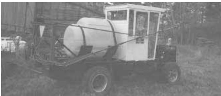
Sprayer was built from a Datsun 4-WD pickup and cab off an IH 300 series combine.
