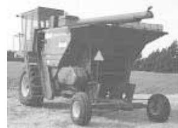
To double the size of the grain tank, he cut the back out and extended it out over the rear axle.
