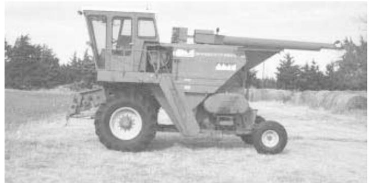
Reinhardt converted this old Massey combine into a self-propelled grain cart by simply doubling the size of grain tank and leaving most of the rest of the machine intact.
