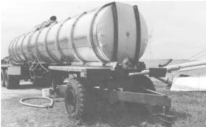
Thomas's trailer uses a conventional 5th wheel mounted on a truck axle fitted with 22-ply airplane tires. Drawbar hitch on front allows trailer to be pulled by a tractor.
