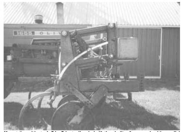
He cut the cultivator's 7 by 7-in. toolbar in half, then built a framework with parallel linkage to lift it with a hydraulic cylinder.
