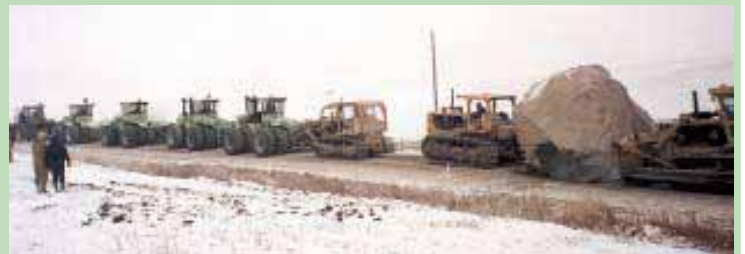
With seven tractors pulling and a D-6 and D-8 pushing from behind (about 3,000 hp in all), they headed down the road - in low gear all around.
