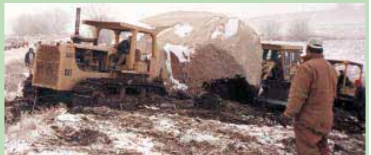
Pushing with their D-6 along with two bigger borrowed Caterpillars, and pulling with a couple of Steigers, they managed to get rock to edge of field in about two weeks.
