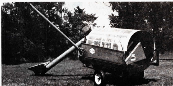
DMC's model 54 cleans 3,000 bu. per hr. and has a 4 in. trash auger for cleanup.
