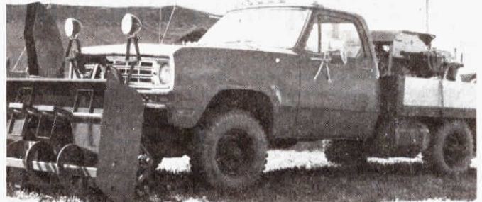
To rig pickups for snowblowing, the company uses hydraulics, mounting an engine and hydraulic motor on the truck bed.
