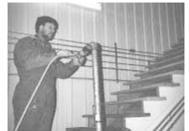
To empty used oil out of reservoir, Smith takes off drain pan and stands unit up straight next to valves by wall. Drain pipe hooks to reservoir (above right). Air hose hooks to fill pipe (below).
