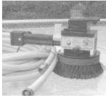
Rotary scrub brush is driven by water pressure from garden hose to create the oscillating motion of a washing machine.
