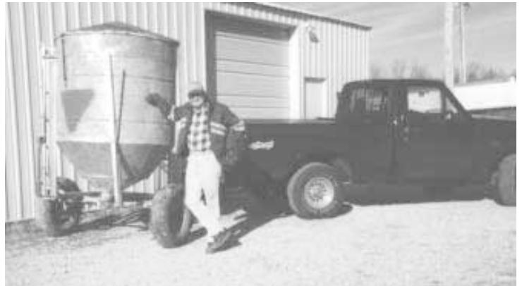
“I use it during the summer to haul ground corn out to my calves on pasture,” says Wilburn Lemons, who mounted a 40-bu. hog feeder on top of a pickup steering axle.
