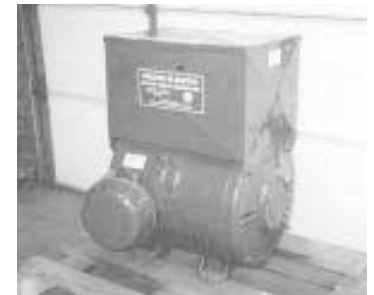
Converter allows you to produce your own 3-phase power from a single phase line.
