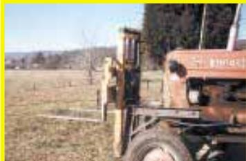
standard forks on it or attach a bale spike in place of them. Hydraulics are supplied by a pump on the right side driven by bolting a flangeless (hubless) V-pulley on the belt pulley hub. The tractor's one-way hydraulics run through 2-way controls mounted on the right fender. **(Harold R. Stoudt, 1241 Hex Highway, Hamburg, Penn. 19526)**
