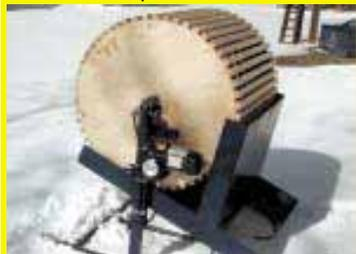
wise at 94 rpm's. The outside tank, with the slats, runs 12 to 14 rpm's. I can shell a peck of nuts in anywhere from 5 to 9 min., depending on the thickness of the shell. It works great. I have shelled 80 bu. in 4 weeks. About 90 percent of the nuts come out in halves. I am applying for a patent on this great new design. **(Hoover A. Lingle, 1022 S. Main GQ St., Salisbury, N.C. 28146 ph 704 279-2465)**
