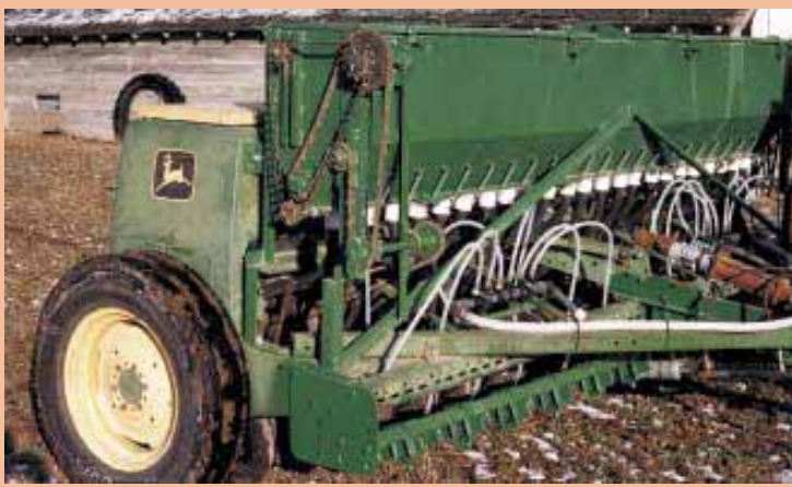
Miller modified his Deere 8200 drill by mounting a fertilizer box on front and adding knives that band liquid urea 3 in. to the side of the furrow and 2 in. below the seed.
