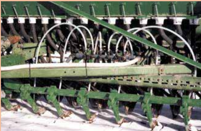
Knives clamp onto a 2-in. sq. toolbar mounted ahead of drill's openers.
