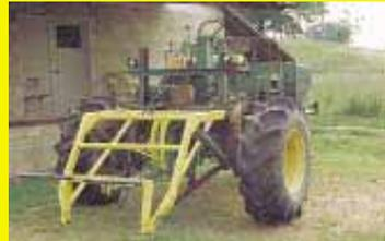
the arms. A hydraulic cylinder mounted behind the frame is used to move the bale up or down and to tilt the bucket.
