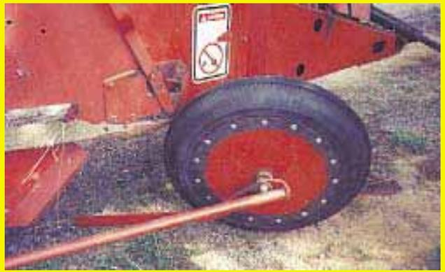
The gathering wheels on my Hesston 5530 round baler were worn out so I replaced them with ones that I made out of an old 15-in. tire. The ground-driven rakes - one on each side - gather hay into a windrow that feeds directly into the baler. The original gathering wheels were star-shaped discs made from a rubber that deteriorated over the years. Each one would have cost \$199.99 to replace.
