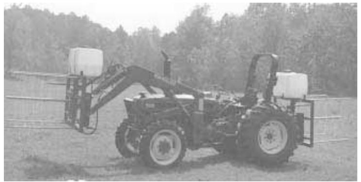
**Tractor-mounted injection system uses 50-gal. reservoir and pto-powered roller pump to inject nutrients into bale. To use, you spear bale and then activate pump to treat it.**
