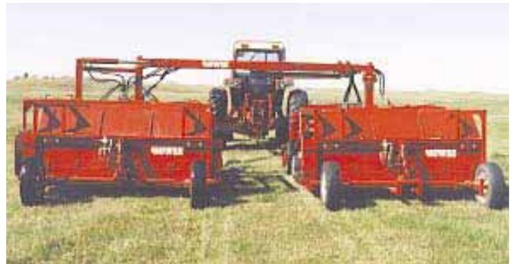
For transport, the tandem hitch pivots backward hydraulically to allow one fluffer to be pulled behind the other.
