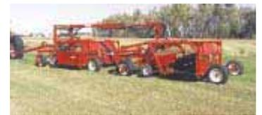
Hitch is designed to pull two 8 or 10-ft. hydraulic-powered hay "fluffers" at the same time.
