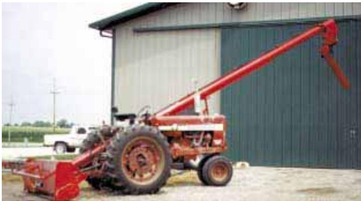
Unit's 8-ft. wide, pto-driven cross auger feeds grain into unloading auger which runs alongside tractor. Auger attaches to 3-pt. hitch and also bolts onto side of tractor.
