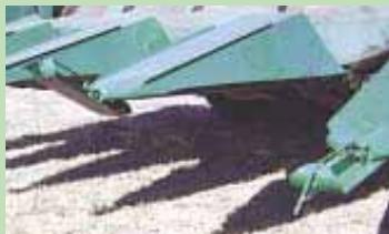
A steel rod angles downward at front of shoe to pick up stalks lying on ground.
