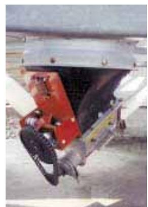
Spring-loaded mallet is chain-driven by a sprocket added to end of unloading auger.
