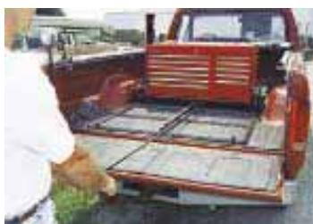
Toolbox rides on a steel track that runs length of bed. A long rod is used to roll it back and forth.
