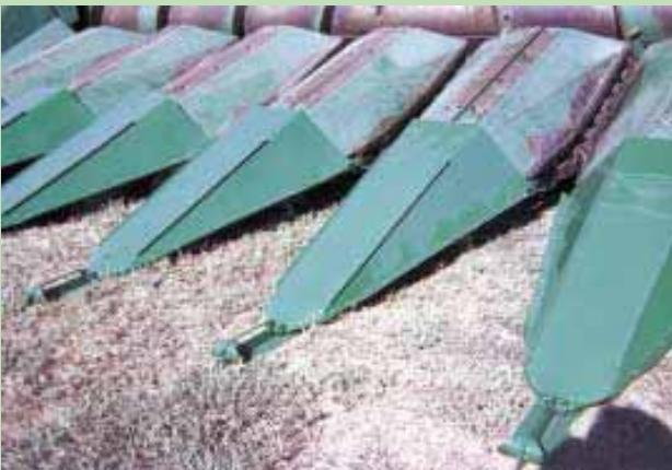
Floating header points bolt on in place of original points and are equipped with a steel shoe that's free to pivot up or down as it slides along ground.
