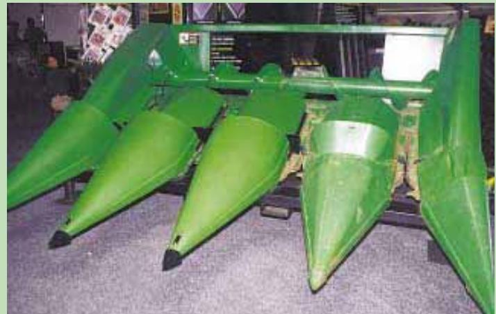
Deere offers these poly snouts for its 40 series heads, made from 1970 to 1993.
